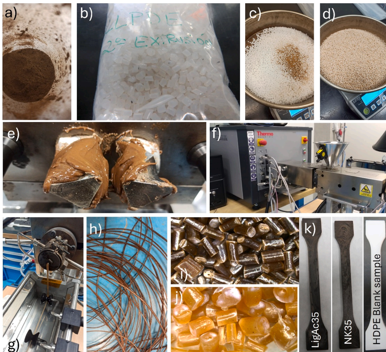
Fig. 1. a) NK powder as received from Creative Nano. b) Neat pellets of commercial PE-Liten-PEHex Polyethylene. c) HDPE and LigAc “as received” materials before and d) after being manually mixed. e) Melted state of the HDPE-LigAc masterbatch within the mixing chamber. f) THERMO FISHER Haake PolyLab QC conical twin screw extruder. g) Compounded filament when being extruded. h) Final filament manufactured. i) and j) final produced pellets from HDPE reinforced with 15 % of LigAc and NK fillers respectively. k) Injected coupons of HDPE containing 35 %wt of LigAc and NK as well as a reference coupon of the neat HDPE polymer.
